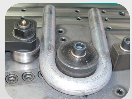
Radial biegen 360° Radial bending 360°
