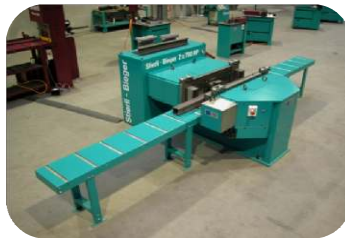
Rohre richten Pipe straightening
